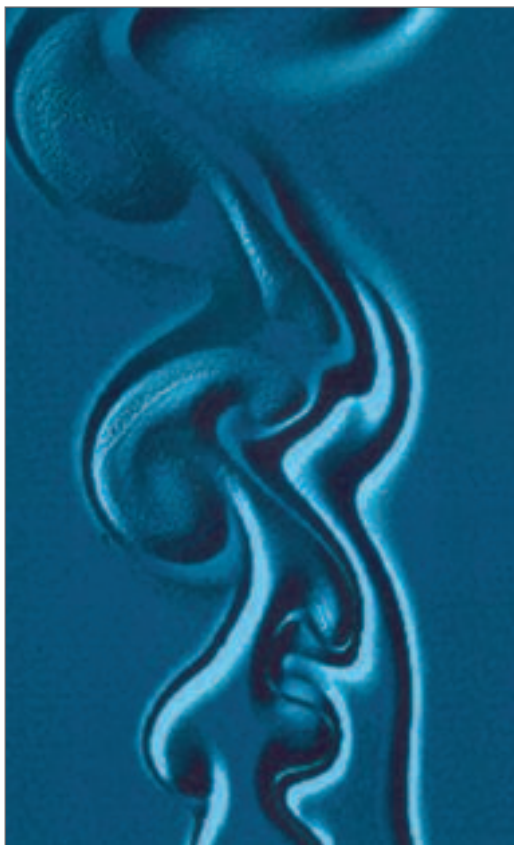
Direct simulation of a mixture of 2 vertical jets at different temperatures
