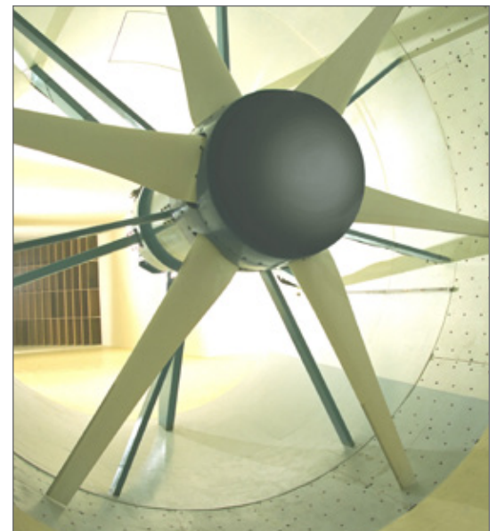
Fan of the concrete wind tunnel
