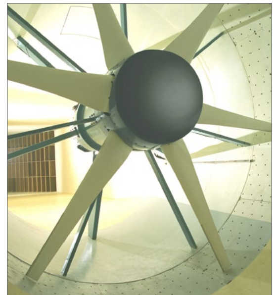
Fan of the concrete wind tunnel
